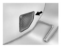
The instrument panel fuse block is located in the center console between the driver and passenger seats. To access the fuses, open the fuse panel door from the passenger side by pulling it out.
